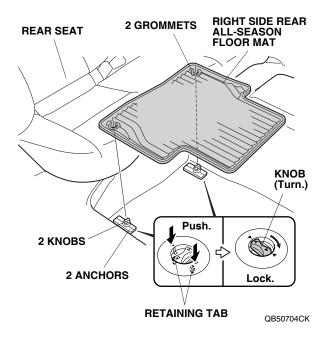
Place the grommets in the left side rear all-season floor mat over the anchors. Push on the grommets into the anchors to secure the retaining tabs, then turn the knobs one quarter turn to secure the allseason floor mat.
