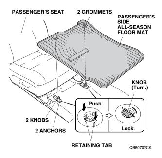
4. Place the grommets in the right side rear all-season floor mat over the anchors. Push on the grommets into the anchors to secure the retaining tabs, then turn the knobs one quarter turn to secure the allseason floor mat.
